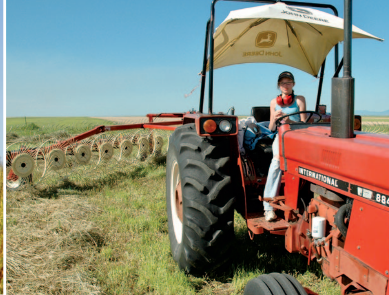
Clockwise from above left: A swather (windrower) cuts hay with a rotating wheel that pulls the plants into a cutter that resembles a long hedge trimmer; to dry hay in wet conditions, a hay rake fluffs and flips the long rows left behind the swather; a round baler rolls the cut crop into rounds that weigh up to a ton; bales are then loaded with hydraulic lifts onto truck trailers or stored in stacks. Bottom: a standard 60-pound hay bale produced by a square baler.
