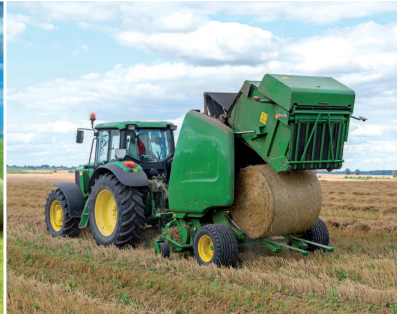
Clockwise from above left: A swather (windrower) cuts hay with a rotating wheel that pulls the plants into a cutter that resembles a long hedge trimmer; to dry hay in wet conditions, a hay rake fluffs and flips the long rows left behind the swather; a round baler rolls the cut crop into rounds that weigh up to a ton; bales are then loaded with hydraulic lifts onto truck trailers or stored in stacks. Bottom: a standard 60-pound hay bale produced by a square baler.
