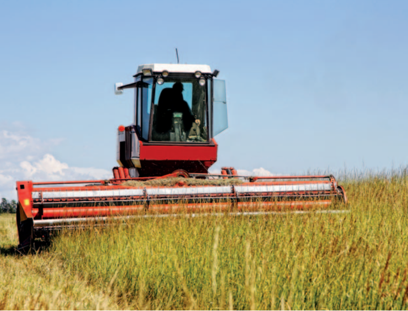
Clockwise from above left: A swather (windrower) cuts hay with a rotating wheel that pulls the plants into a cutter that resembles a long hedge trimmer; to dry hay in wet conditions, a hay rake fluffs and flips the long rows left behind the swather; a round baler rolls the cut crop into rounds that weigh up to a ton; bales are then loaded with hydraulic lifts onto truck trailers or stored in stacks. Bottom: a standard 60-pound hay bale produced by a square baler.
