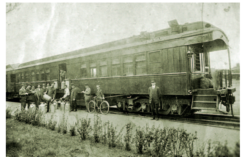
TROUT TRACKS From 1871 to 1940, the U.S. Fish Commission delivered brown trout and other fish on specially designed train cars to Montana and other states, as well as to private groups and individuals. The cars had water tanks, aeration devices, cooling systems, and bunks for the attendants. Recipients would wait at the station to pick up fish and stock them into local rivers or ponds. In 1940, the commission was abolished when it became part of the newly created U.S. Fish & Wildlife Service.
