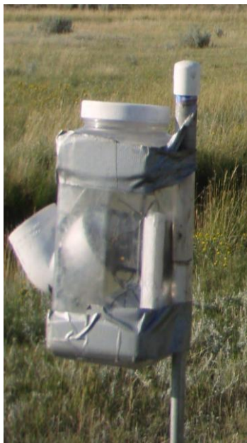
Figure 7. Photograph of a bat acoustic detector sampling site, showing an iRiver H320 recording unit housed inside a protective enclosure that is mounted to a pipe.
