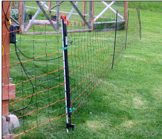
Figure 3. Portable temporary electrified net fence, positive/negative design
