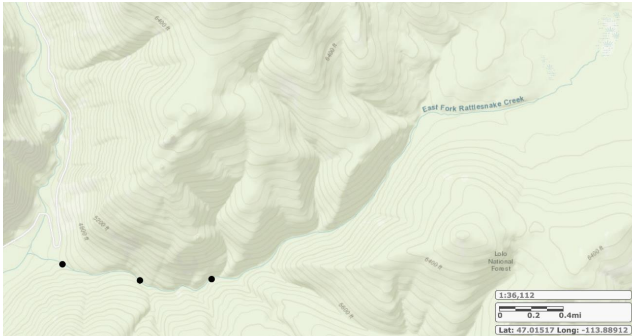
Figure 1: A hypothetical distribution of sampling in a first order tributary. Note that sampling is dispersed across three reaches that are >500m apart.
