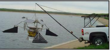
Hoisting SolarBee Out Of Water
