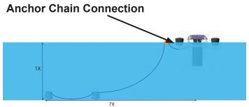
SolarBee Anchored With Mooring Block System
