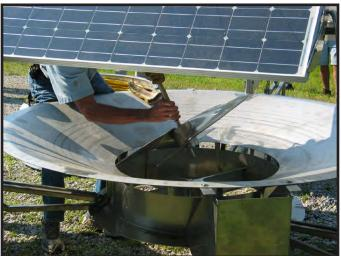
Impeller Removal For Buildup Below Impeller
