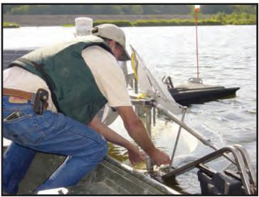
Hooking Depth Indicator Chain Into Slot
