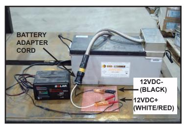
12 VDC Battery Charge Setup
