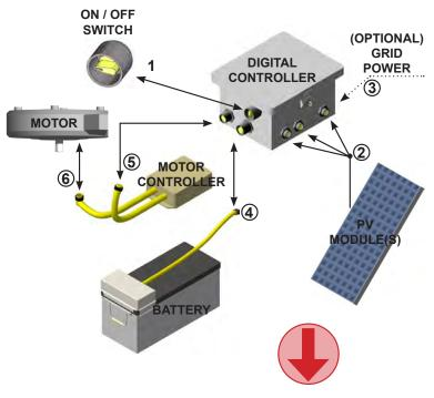
WARNING: ONCE BATTERY IS CONNECTED TO BATTERY ADAPTER CORD, DO NOT ALLOW WHITE AND BLACK CONTACTS TO TOUCH ONE ANOTHER OR IT WILL RESULT IN A DEAD BATTERY SHORT AND SPARKS WILL BE EMITTED. USE EXTRA CAUTION TO PREVENT A DEAD SHORT WITH BATTERY OR CHARGER.
