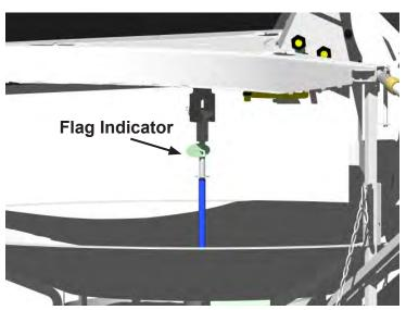
Flag Indicator Section of Impeller Shaft
