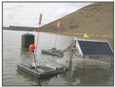
Anchor Chain Connection Point (At Float Ball)
