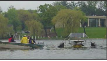
Towing SolarBee Using Small Boat
