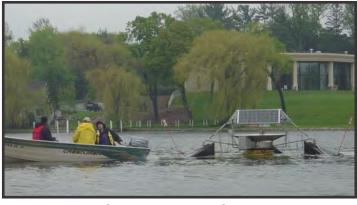
Towing SolarBee Using Small Boat
