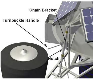
Water Level Even With Notch On Chain Bracket
