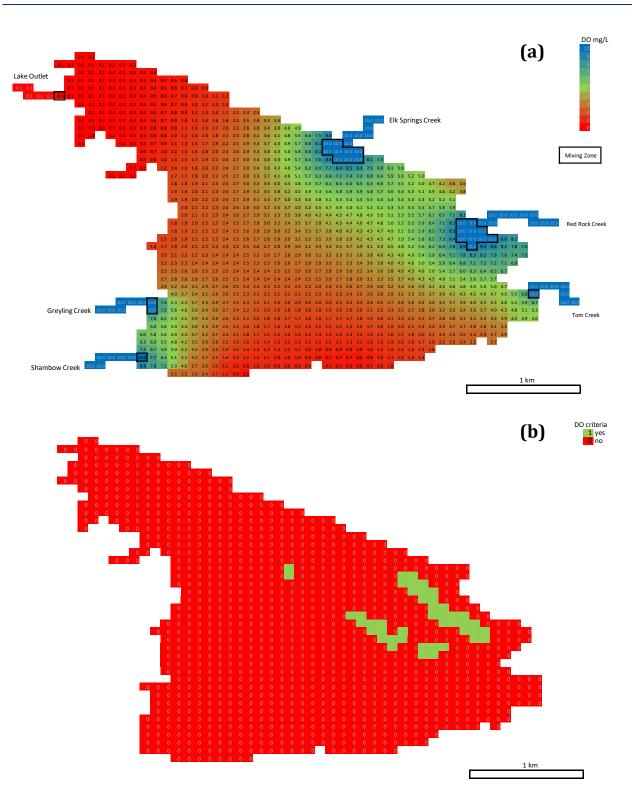
Figure 6-42-D Modeled Response of URRL to the dredging alternative(a) Predicted oxygen concentrations. (b) Predicted winter habitat area.
