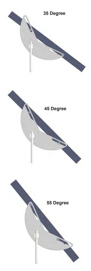
For cable tethered anchoring, the north facing panel may be flipped to face the south using a special panel gate. A tethered machine is fixed and will not rotate, so the north facing panel will receive the least sunlight, unless flipped using the special gate. For mooring block anchoring, this is not an option due to the machine rotating about the mooring blocks.
