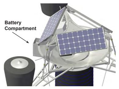
**Onboard Battery** - The onboard battery is located directly below the dish in a stainless steel compartment. During operation, the battery is submerged in the water to maintain a stable-temperature environment that increases its performance and life. The battery is double-walled to isolate its contents from the water it is submerged in.
