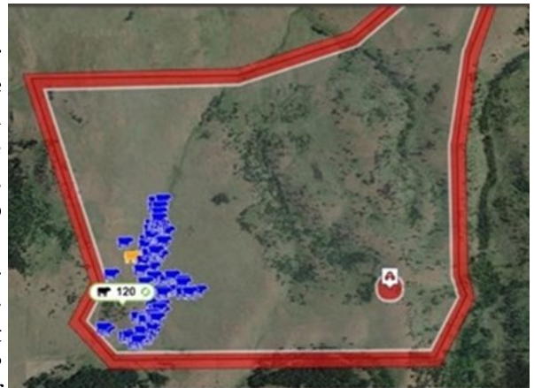
Above: Vence's collar management program (Herd Manager) provides a visual representation of the virtual fence polygon (red). In this scenario, each collar (or cow) is displayed as a blue or yellow cow icon on the screen. Virtual fence boundaries can be adjusted via the Herd Manager program. Below: Location data points for all collared cows for the first 30 days they were on the WMA appear in this figure. Some cows breached the virtual fence boundary.
