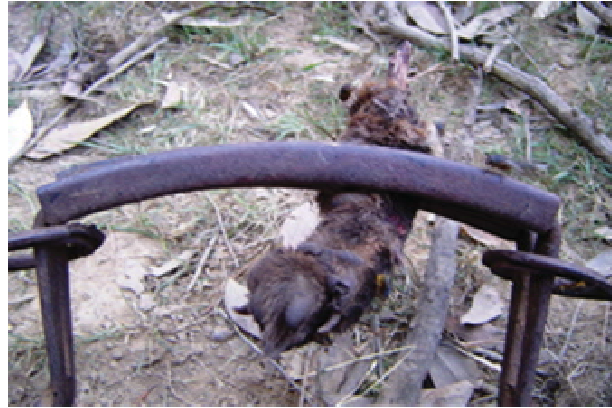
Figure 12. Older styled (modified) long-spring leg-hold traps are substantially heavier and have a larger ‘jaw spread’ than many contemporary (coil spring) leg-hold trap devices. Their weight and tendency to catch animals higher on the leg appears implicated in increased fractures and amputations.
