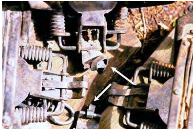
Figure 5. Damage to 'Paws-I-Trip' ® pan tension device 'dogs' caused by chewing (indicated by arrows) of the Victor Soft-Catch #3 traps after capture of dingoes (after Marks et al. 2004).
