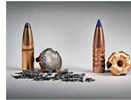
FULLY INTACT Comparison of a copper-jacketed lead bullet and fragments after firing into water jugs, and a polymer-tipped all-copper bullet that retained 100 percent of its mass in the same test.
