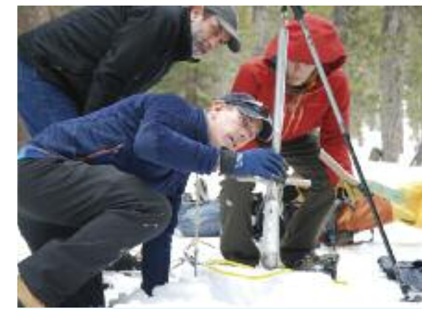
WATER FORECAST Backcountry snow surveyors follow set courses, using corers and scales invented by James E. Church in the early 1900s to sample snowpack.
