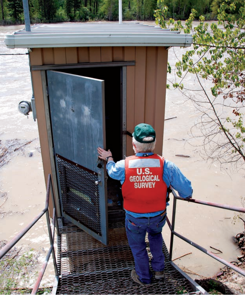
CURRENT AFFAIRS Clockwise from above left: “Lucky” Sultz, a retired streamgager, enters a gagehouse on the Flathead River at Columbia Falls where river stage is automatically recorded every 15 seconds and transmitted by satellite to U.S. Geological Survey offices. Streamgager Phil Karper pulls his cable car across the Missouri River near Great Falls while testing current velocity. Greg Trunkle lowers a small tri-hulled boat outfitted with Doppler radar into the Flathead River. The high-tech electronics are used where rivers allow bridge access. Without bridges, streamgagers use cable cars and lower a torpedo-shaped weight fitted with a device (white arrow) that measures current velocity as it spins.
