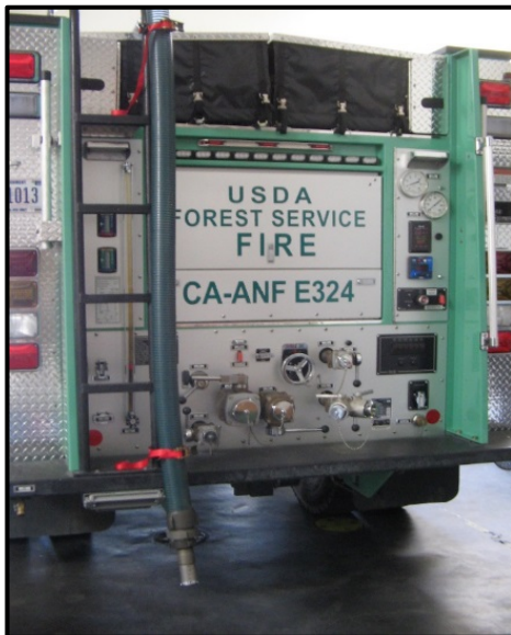
Figure 8 Suction hose with foot valve attached to engine ladder.
