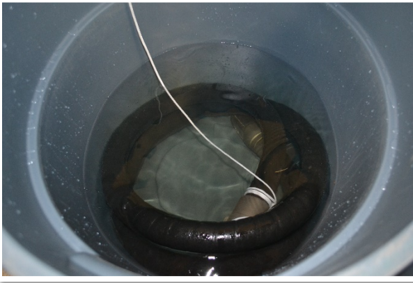
Figure 4: Draft hose fully submerged in chemical solution
