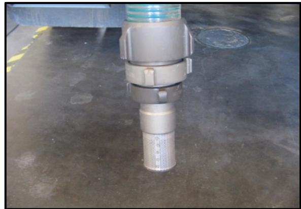
Figure 9. Foot valve attached to suction line with various adapters as needed to adjust for foot valve size.
