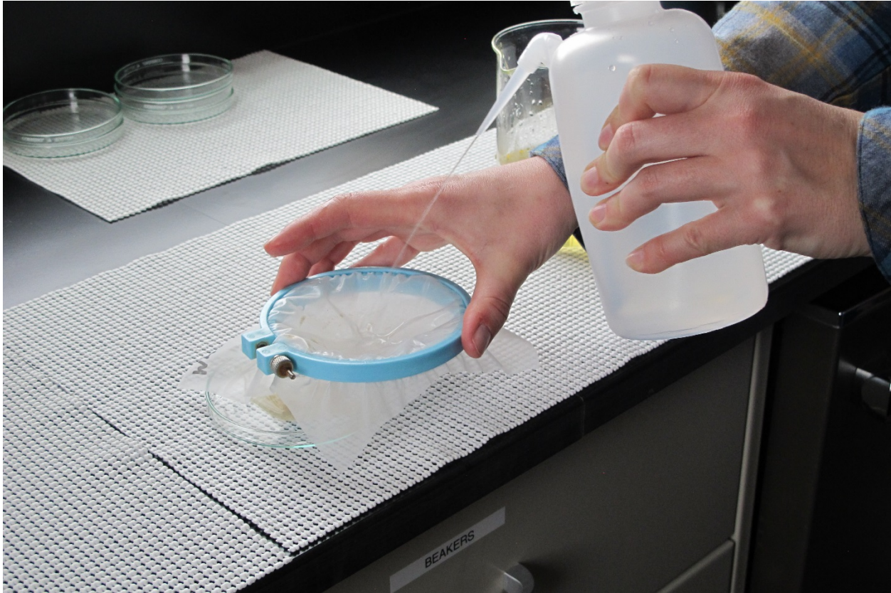
Figure 25: Rinse contents of 35 µm filter into glass Petri dish. More than one Petri dish should be used for samples with high algae or sediment content.
