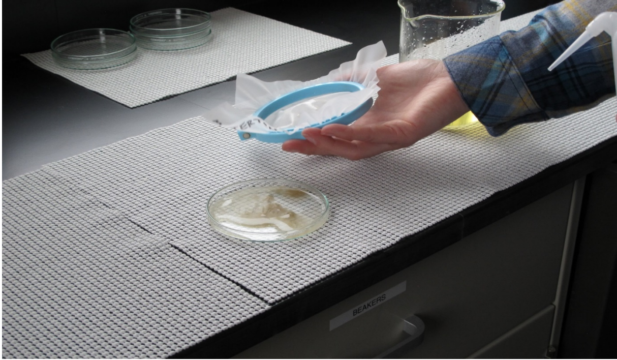
Figure 26: Use DI wash bottle and gentle agitation to separate clumps of particulate matter.
