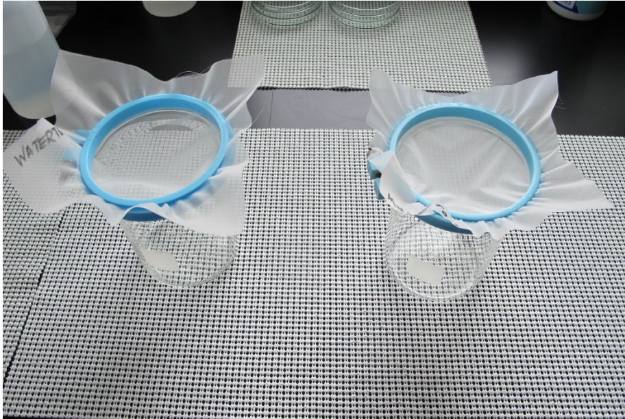
Figure 20: Set up two beakers with 210 and 35 \mu m filters.
